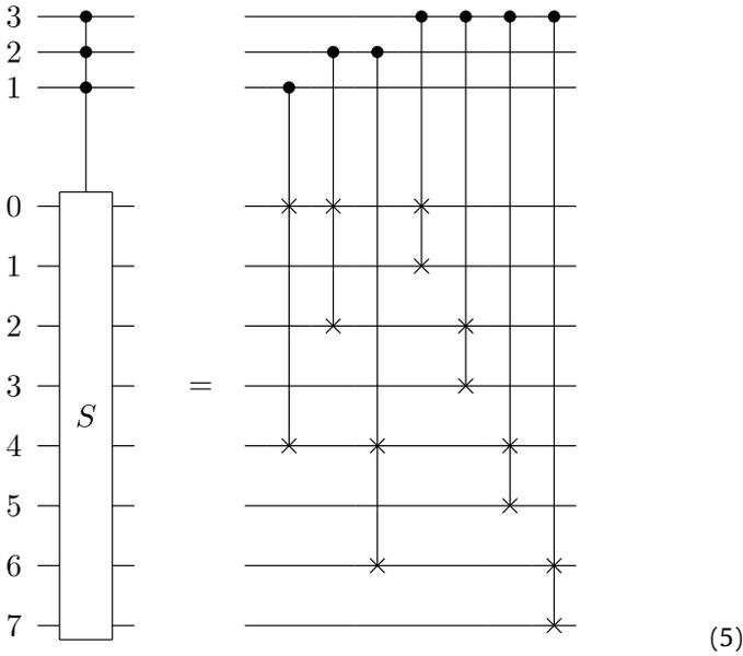
The result of Theorem 1 allows us to conclude that Task 1 is achievable by an ordinary quantum circuit on  $\mathbf{O}(N \log N)$  ancillary qubits plus 1 system qubit, and resorting to  $\mathbf{O}(N^2)$  elementary operations, as follows
