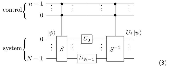
In the circuit, the system register is prepared in the state  $|\psi\rangle \otimes |0\rangle^{N-1}$  and the control in the state  $|[i]_n\rangle$ . This will output the state  $U_i|\psi\rangle$  on the first system qubit. For this purpose one first operates an  $n$ -controlled swap  $S$ , then each system qubit  $i$  undergoes  $U_i$ , and finally an inverse  $n$ -controlled swap  $S^{-1}$  is made. The  $n$ -controlled swap is achieved by the following circuit:
