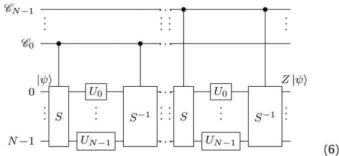
where  $Z = U_{i(N)} \dots U_{i(1)}$  denotes the programmed disposition of unitaries, and  $\mathcal{C}_i$  ( $i = 1, \dots, N$ ) denote a control register made of  $n$  qubits. The circuit is just the juxtaposition of  $N$  copies of circuit (3),  $\mathcal{C}_i$  being the control system of the  $i$ th circuit.
