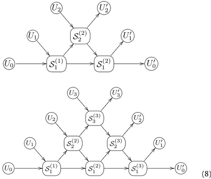
It is easy to see that the circuit uses overall  $\sum_{n=1}^{N-1} n = \frac{1}{2}N(N - 1)$  QSS, each with a single-qubit control register.
