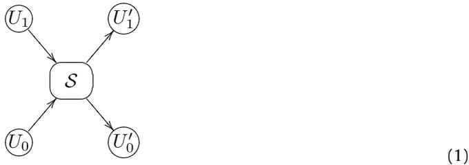
where  $S$  represents the QS having two inputs and two outputs,  $U_0$  and  $U_1$  denote the two input unitary channels, and  $U'_0$  and  $U'_1$  are the two output ones, which are either  $U'_0 = U_0$  and  $U'_1 = U_1$  or  $U'_0 = U_1$  and  $U'_1 = U_0$ , depending on the state  $|0\rangle$  or  $|1\rangle$  of a control qubit  $s$  (not represented). In formula
