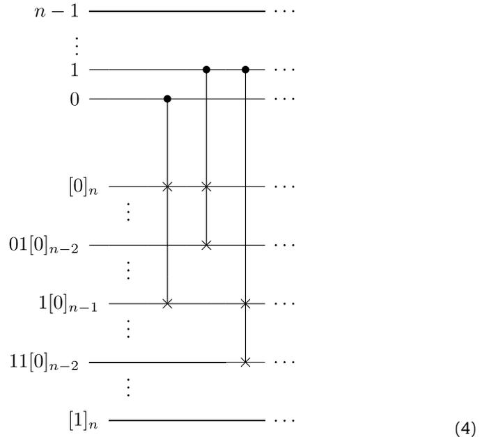
In words, for  $k = 0$  to  $n - 1$  the circuit does the following: insert  $2^k$  control-swaps controlled by the  $(k + 1)$ th control qubit and swapping system qubit  $[s]_k[0]_{n-k}$  with system qubit  $[s]_k[1]_{n-k-1}$  for every  $k$ -bit string  $[s]_k$ .
